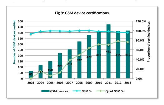
The incidence of quad-band GSM remained stable at 76 per cent in 2013. 81 per cent of all devices (355 devices) incorporated EDGE.
